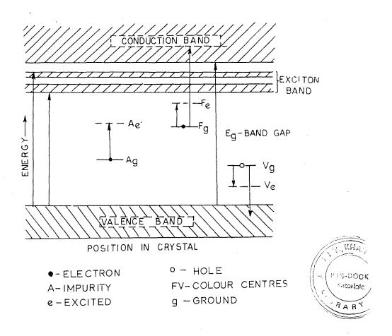
FIG. 1.1 BAND PICTURE OF AN ALKALI HALIDE, SHOWING ENERGY LEVELS AND SOME OPTICAL ABSORPTIONS DUE TO EXCITONS, IMPURITIES AND COLOUR CENTRES (SCHEMATIC)
