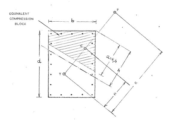
C = TOTAL COMPRESSION IN STEEL AND CONCRETE
