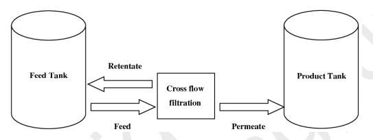
Figure 1.2: Schematic illustration of cross-flow filtration
