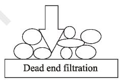
Figure 1.1: Schematic illustration of dead end filtration
