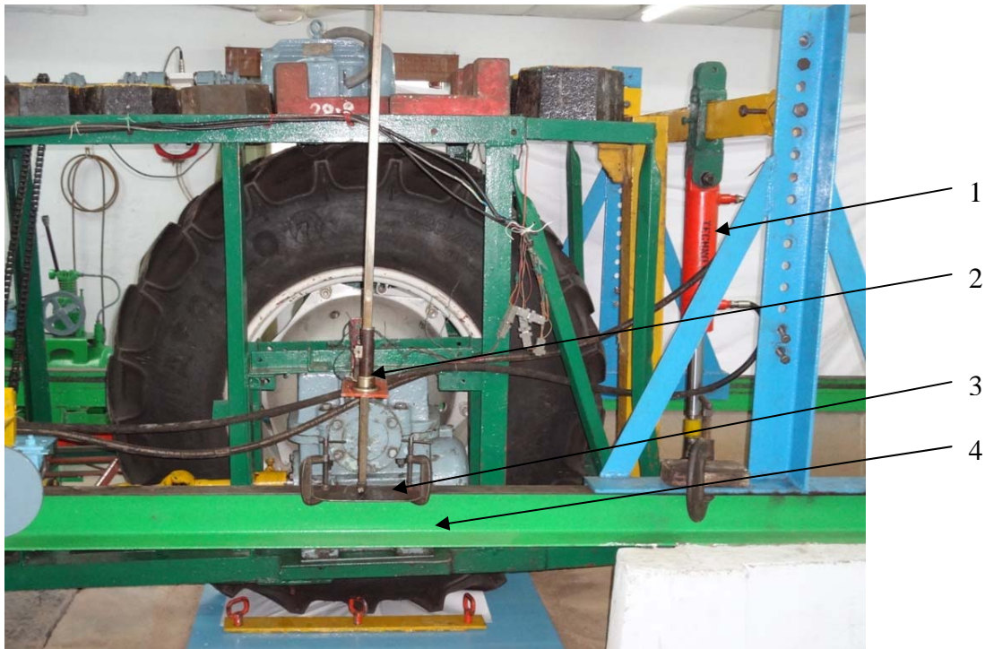
1. Hydraulic cylinder 2. Displacement transducer 3. Base plate 4. Side rail
