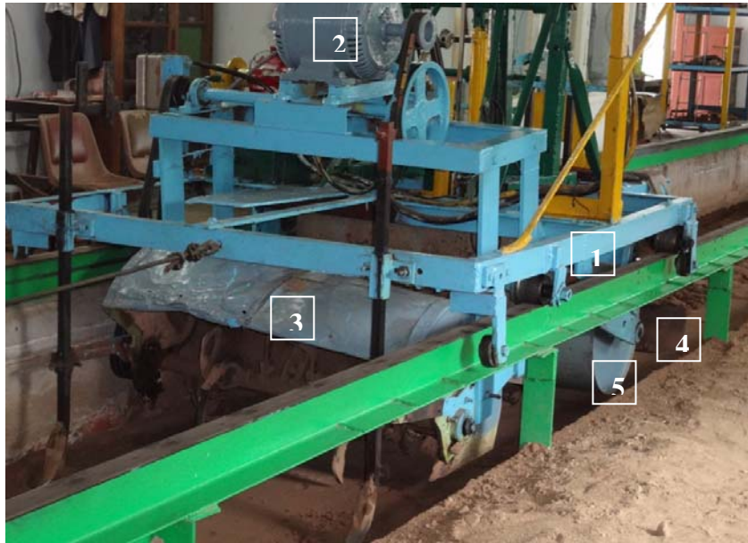
1. Main frame 2. Induction motor 3. Soil tiller 4. Soil leveler 5. Soil compacting roller
