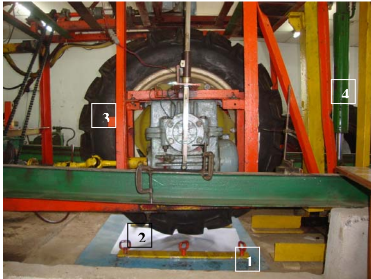
1. Steel plate 2. white sheet 3. Test tyre 4. Hydraulic cylinder Fig. 4.6 Set-up for measurement of tyre-ground contact area
