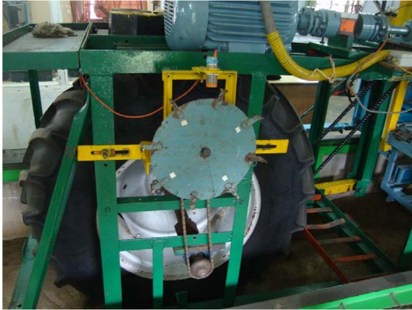
Fig. 4.20 Theoretical forward speed measuring device
