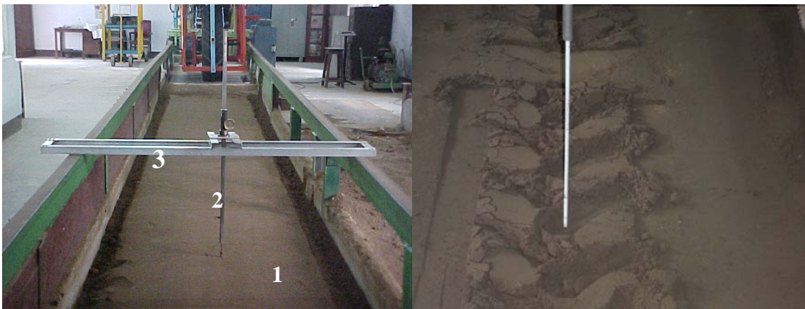
Fig. 4.21 Tyre sinkage measuring device
