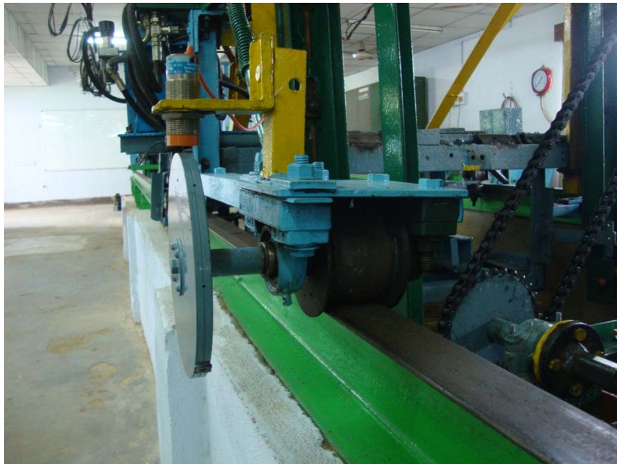
Fig. 4.19 Actual forward speed measuring device
