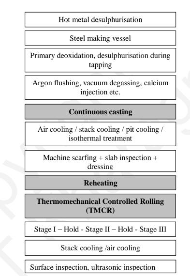
Fig. 1.1.2: Flow chart showing the typical processing route for TMCR-microalloyedpipeline steels. The dark shaded stages are important from the point of view of grain structure and therefore, are studied in the present investigation to follow the changes in grain size [Gray, 1983].
