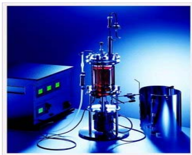
Fig. 1.9: A Continuous Stirred Tank Reactor
