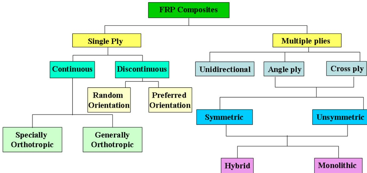
Fig. 1.1: Classification of Fibre Reinforced Plastic (FRP) composites.
