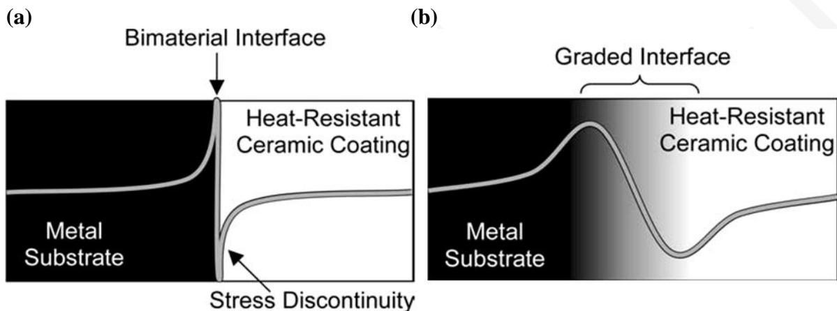
Fig. 1.3: (a) Stress concentration at the bimaterial interfaces, overcome through (b) smooth transition of material properties through the graded interface of the FGM.
