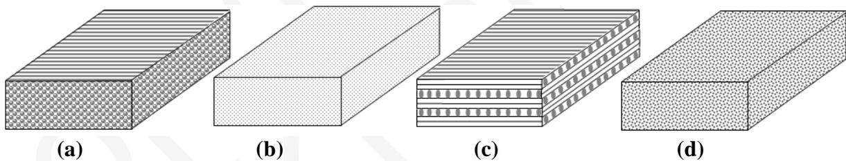
Fig. 1.2: Various types of polymeric composites (a) Fibrous, (b) particulate, (c) laminated, and (d) flake.
