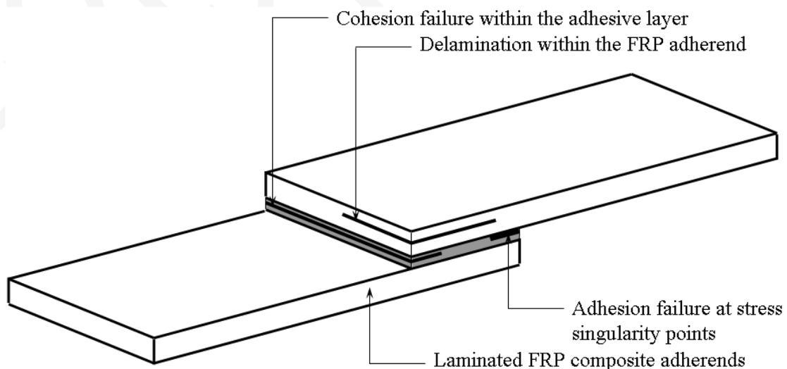
Fig. 1.5: Prominent failure modes in an adhesive bonded single lap joint made with laminated FRP composite adherends.
