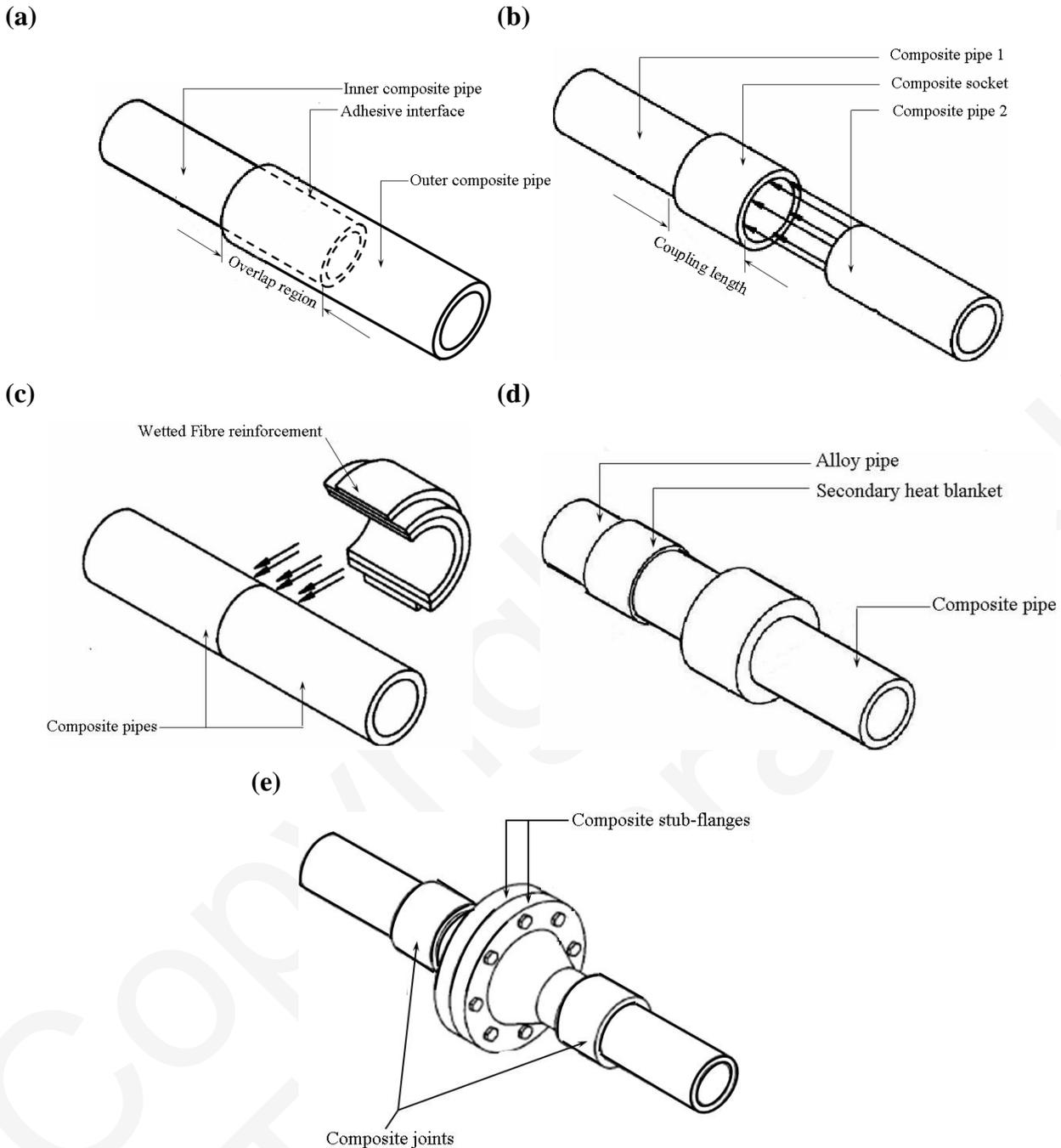
Fig. 1.6: Different types of joining methods used in the composite piping systems: (a) Single lap joint, (b) Socket joint, (c) Butt-and-strap joint, (d) Heat-activated coupling joint, and (e) Flanged joint.
