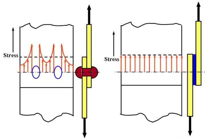
Fig. 1.4: Comparison of stress distribution in (a) mechanically fastened joint and (b) adhesive bonded joint.
