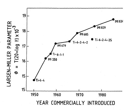
FIG. 11: CREEP RESISTANT TITANIUM ALLOY DEVELOPMENT:
