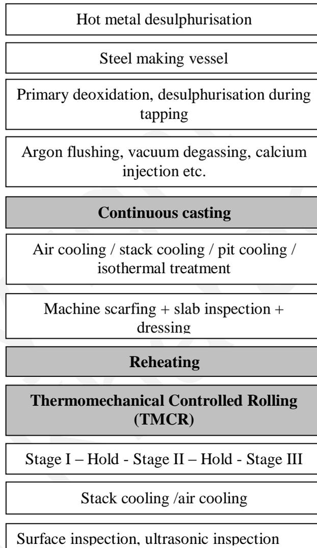
Fig. 1.1.2: Flow chart showing the typical processing route for TMCR-microalloyed-pipeline steels. The dark shaded stages are important from the point of view of grain structure and therefore, are studied in the present investigation to follow the changes in grain size [Gray, 1983].
